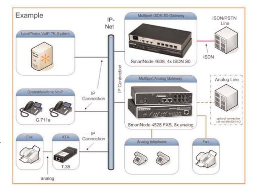
Asterisk-based phone systems rely on internal PCI cards (installed within the Asterisk server) to connect to ISDN or analog networks. LocaNet, however, has selected SmartNode™ VoIP Routers for deployment as external media gateways. But why?
