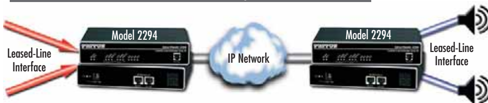
The 2292 and 2294 extend leased lines over any IP network
