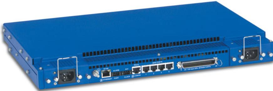
The Model 3092 ISDL Digital Access and Cross-Connect System (DACS) is the efficient, rack-mountable solution for ILECs/PTTs expanding their access services via ISDL dedicated links. The Model 3092 combines ISDL ports for concentration to multiple TDM WAN ports with total flexibility in mapping the ISDL channels and WAN time slots. The Model 3092 is extremely reliable due to its convection cooling (with no fans or other moving parts to fail) and dual-redundant power supplies.
