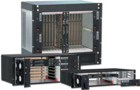
The Patton ForeFront™ 6500 Series DACs are carrier grade digital cross connects with unparalleled redundancy and upgradeability. Whether used as a cross connect or a multiplexer for TDM aggregation, ForeFront DACs are flexible, rugged and easily upgradeable.
