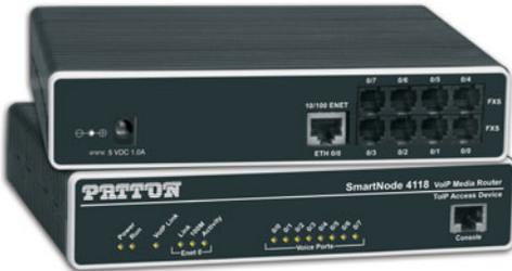
The SmartNode 4110 VoIP Media Gateway supports up to eight transparent phone calls while leveraging VoIP for lower-cost carrier and corporate access. Connecting to any analog phone, fax, or PBX, the SN4110 is an effective and flexible solution for toll-bypass, remote/branch office voice connectivity, and enhanced carrier services.
