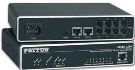
The EtherBITS family of device servers provide easy, feature rich, secure and reliable serial to LAN, WAN or Internet connectivity. Placing serial devices on to the LAN eliminates the hassle of serial cables, dedicated PCs, and local management. Providing Ethernet connectivity to your serial devices not only protects your current hardware investments, but simplifies future expansions and the management of that hardware.
