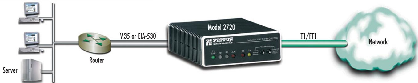
The Models 2720 and 2710RC T1 CSU/DSUs come with V.35 or EIA-530 for simple connection to routers or multiplexers at the customer or service provider premises. The 2720 and 2710RC
