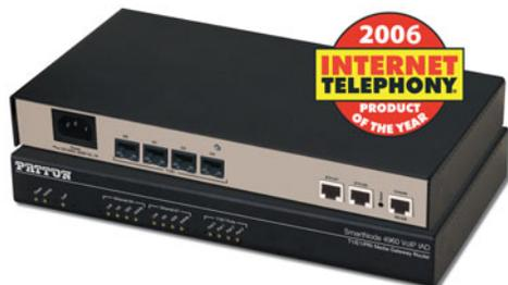
Providing a high-density seamless link between the circuit-switched telephone network and voice-over-IP, the SN4960 is ideal for PBX business trunking or corporate VoIP access. Offering up to four software configurable T1/E1/PRI interfaces the SN4960 connects to any switch, PBX and data network with up to 120 simultaneous calls using SIP, T1, E1 or PRI signaling. The dual gigabit Ethernet ports connect to the network for the highest throughput with its integrated QoS router. With
