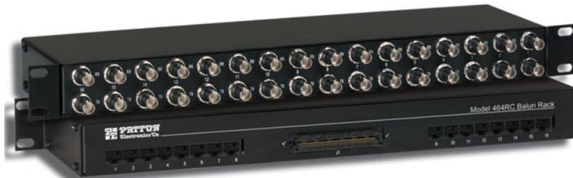
The Patton 464RC & 466RC G.703 balun panels match 16 sets of dual 75-ohm coax connections to 120-ohm twisted pair connections. This function allows carriers to provide 120-ohm G.703 service to customers retaining 75-ohm CPE hardware. It also allows carriers who have standardized on 75-ohm coax to provide 120-ohm terminations to their customers (in keeping with European ONP requirements).
