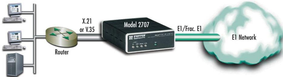
The Model 2707/D (X.21 version) provides DTE/DCE functionality in the same standalone or rack-mount package. This added versatility supports operation in X.21 DTE applications (see diagram above) where an NTU is needed to terminate G.703 and provide X.21/V.11 data to a multiplexer.
