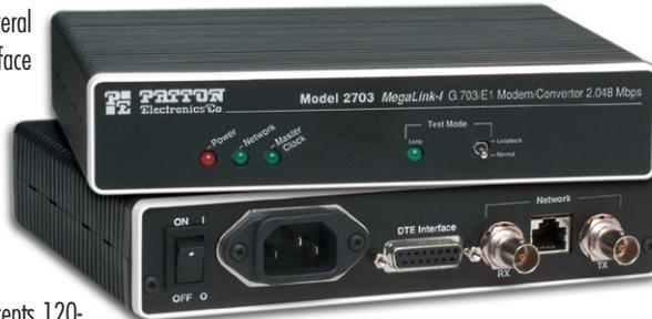
a 2.048-Mbps G.703 link. The Model 2703 supports internal, external or network (receive loop) clocking. A loopback test is built-in, and front panel LEDs monitor power, network, master clock and test loop. Several power supply options and convert-er cables are available, call for details.
