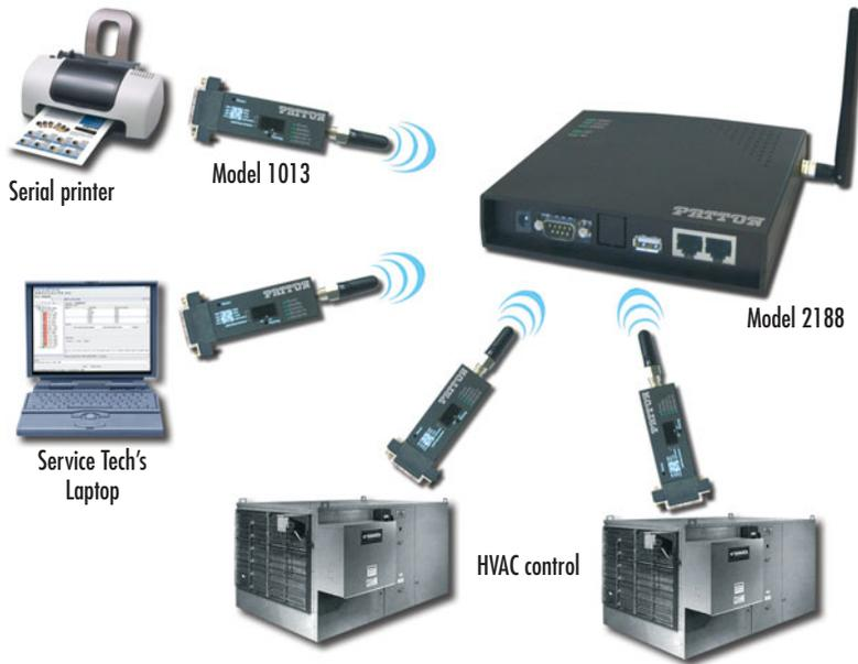
Bluetooth enables wireless RS-232 connections, making installations and service calls more efficient by eliminating the time, hassle, and expense of cable runs.
