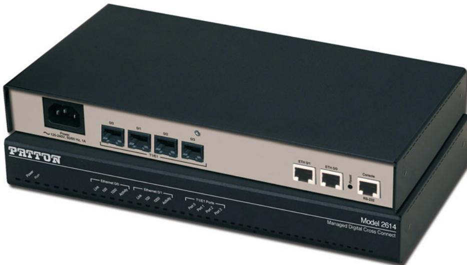
The Model 2614 Managed Digital Cross Connect is the ideal low-cost solution for cross connecting and multiplexing DSOs for up to 4 T1/E1 ports. A good choice for both enterprises and service providers needing to groom and optimize data bearing circuits, the Model 2614 comes in a sleek, desktop package for easy installation in almost any environment.
