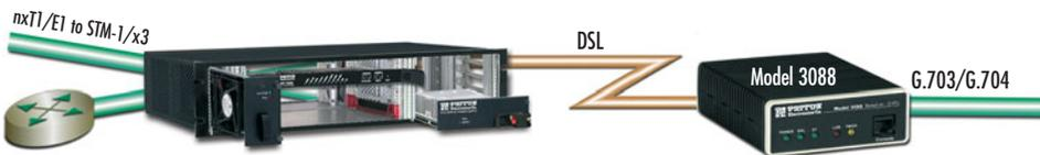
Using ForeFront with the Model 3088 allows deployment of hundreds of DSL circuits from a single low profile chassis. The Model 3088 can be used on the customer premise to deliver T1/E1 co-directional G.703, X.21, or V.35 interfaces.
