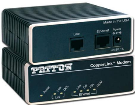
The Patton Model 2168 Multi-Rate CopperLink Ethernet Extender enables the utilization of existing copper infrastructure for high speed Ethernet extensions at data rates up to 16.67 Mbps. The Model 2168 Ethernet Extender includes seven asymmetrical and symmetrical settings which provide the flexibility to increase the distance or speed of the Ethernet connections.
