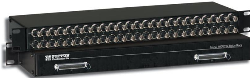
The Patton 450RC24 G.703 balun panel matches 24 sets of dual 75-ohm coax connections to 120-ohm 50-pin telco connections. This feature allows network & datacom equipment manufacturers who are selling equipment for use in COs with only 120-ohm telco interfaces to offer their equipment to G.703 countries using 75-ohm connections. This eliminates the mismatch with coax legacy equipment in many COs.
