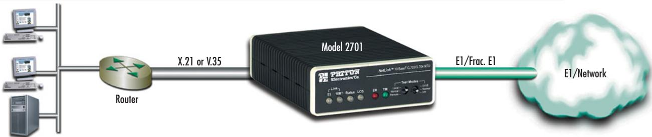
The Model 2701/D (X.21 version) provides DTE/DCE functionality in the same standalone or rack-mount package. This added versatility supports operation in X.21 DTE applications (see diagram above) where an NTU is needed to terminate G.703/G.704 and provide X.21/V.11 data to a multiplexer.
