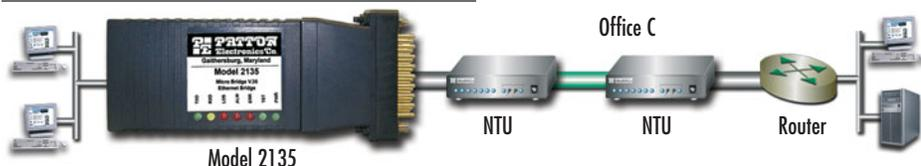
Patton's Ethernet MicroBridge Series are compliant with the RFC 1661 standard for PPP half-bridging, so you can connect our bridge to a router (instead of another bridge) which saves you money!
