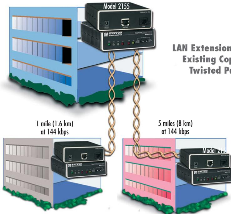
**LAN Extension Using Existing Copper Twisted Pair**
