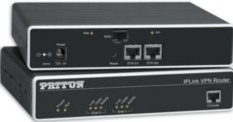
The ILink™ G.SHDSL.bis VPN Router is a next generation business-class G.SHDSL router that addresses both the security and the traffic prioritization needs of enterprises while providing complete broadband integration with existing DSLAM networks. VPN routers enable the secure communication between remote offices, home offices, and mobile users across insecure IP networks such as the Internet. The 3210 takes it one step further and integrates quality of service (QoS).
