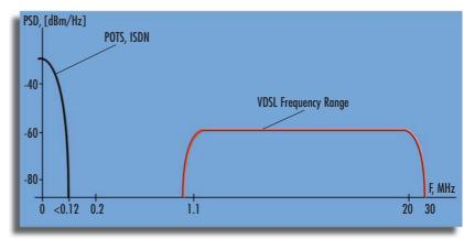
Frequency Division Multiplexing (FDM) allows one pair of wires to simultaneously transport data (VDSL) and voice (POTS/ISDN) traffic. The lower frequencies are reserved for voice (POTS/ISDN) and the higher frequencies for data (VDSL).
