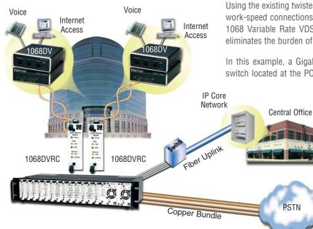
Using the existing twisted-pair voice-grade copper infrastructure to deliver network-speed connections up to 16 Mbps is now possible using Patton's Model 1068 Variable Rate VDSL Modems. Using the existing copper infrastructure eliminates the burden of installing and absorbing CAT-5 and fiber costs.
