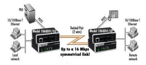
Used in pairs (Central Office and Customer Premise), the Model 1068 establishes a high-speed, line sharing, asymmetrical or symmetrical voice and data link. The Model 1068 inter-connects two geographically separated LANs over a voice-grade twisted pair wire.
