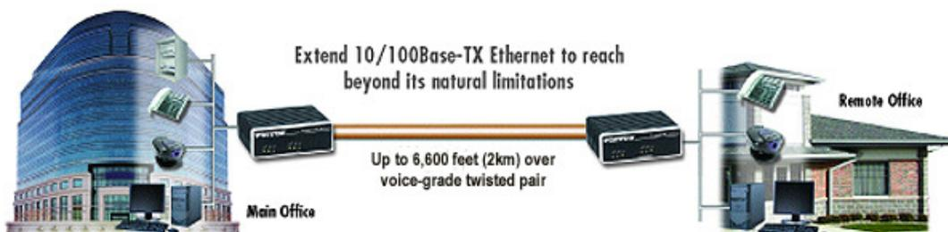
Used in pairs, the Patton Model 2168 establishes a high-speed (up to 16.67Mbps) communications link inter-connecting two geographically separated LANs or network enabled devices. Operation is simple: packets destined for the remote LAN are sent transparently, at full line rate, to the peered LAN. CopperLink Ethernet Extenders utilize ordinary voice-grade wire thus eliminating the cost and common barriers associated with installing new cable or expensive fiber.
