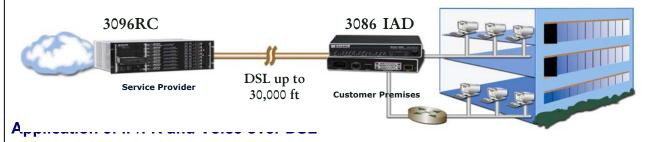
Patton's Model 3086 can also connect to a PBX – In addition to providing IP/FR/ATM/PPP connectivity for a 10/100 Ethernet LAN, the 3086/RIK's drop-and-insert port connects to a local PBX to provide voice and
