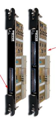
Rear access cards provide any-to-any DSO connectivity. Additionally, it provides 4, 8, 12, or 16 E1 WAN egress ports.
