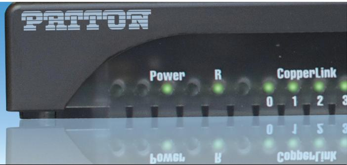
The CL2300 offers the best bandwidth and distance combination in the CopperLink product line. Speeds in excess of 22.8 Mbps symmetrical at distances of 2 miles are possible due to Patton's pair bonding which supports up to 4 individual twisted-pairs (8-wire) or just a single Cat 5 or higher rated cable.
