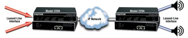
Patton SmartNode Models 2292 and 2294 are equipped with two Ethernet ports and provide gateway and Voice-over-IP line extension services.
