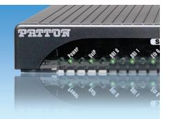
The SmartNode DTA (Digital Terminal Adapter) is a VoIP Gateway that connects ISDN terminals on one or two BRI/So ports, and converts up to 4 concurrent voice or fax calls to SIP or H.323.
