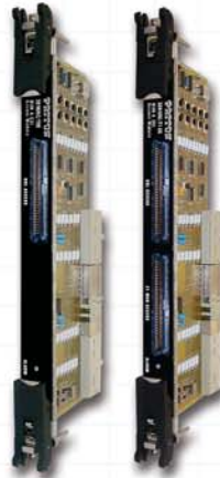
Rear transition modules with flexible interface capabilities
