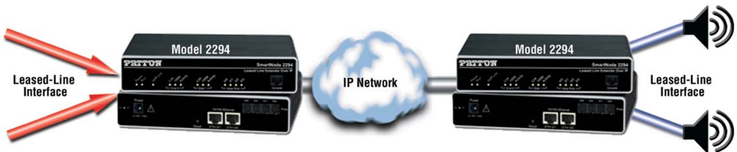
Patton SmartNode Models 2292 and 2294 are equipped with two Ethernet ports and provide gateway and Voice-over-IP line extension services.
