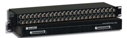
The Patton 450RC24 G.703 balun panel matches 24 sets of dual 75-ohm coax connections to 120-ohm 50-pin telco connections. This feature allows network & datacom equipment manufacturers who are selling equipment for use in COs with only 120-ohm telco interfaces to offer their equipment to G.703 countries using 75-ohm connections. This eliminates the mismatch with coax legacy equipment in many COs.
