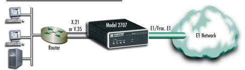
The Model 2707/D (X.21 version) provides DTE/DCE functionality in the same standalone or rack-mount package. This added versatility supports operation in X.21 DTE applications (see diagram above) where an NTU is needed to terminate G.703 and provide X.21/V.11 data to a multiplexer.
