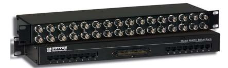
The Patton 464RC & 466RC G.703 balun panels match 16 sets of dual 75-ohm coax connections to 120-ohm twisted-pair connections. This function allows carriers to provide 120-ohm G.703 service to customers retaining 75-ohm CPE hardware. It also allows carriers who have standardized on 75-ohm coax to provide 120-ohm terminations to their customers (in keeping with European ONP requirements).
