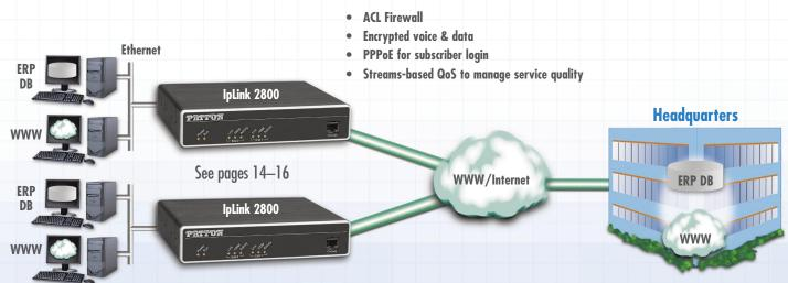
The 2800 series is a line of Enterprise Class Internet Routers supporting a full suite of IP Routing and VPN network functionality
