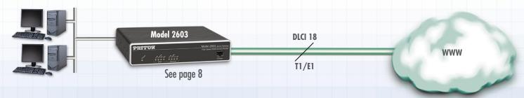
The Model 2603 T1/E1 Router provides basic IP access across T1/E1 lines.
