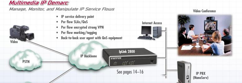
If you are a Carrier using the new IP access network as your "last mile access" to customers and you need a service level demarcation point to terminate your services, the 2800 series is right for you. By establishing differential Quality of Service metrics for voice, data and video services the 2800 series allows the Carrier to manage and control IP
