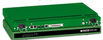
The Model 2688 access router is optimized to process Frame Relay and PPP encapsulated IP traffic from multiple channelized T1/E1 interfaces. The Model 2688 is available in 4, 8, 12 and 16 T1/E1 port configurations with dual 10/100Base-T Ethernet ports. Take advantage of multi-link PPP to grow a link from single to multiple DSOs, all the way to multi-T1/E1 links for the most bandwidth hungry applications and services.
