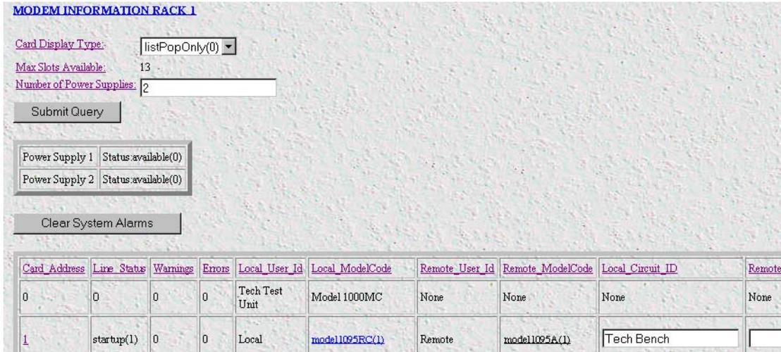
Figure 42. Modem Information page for the Model 1095RC
