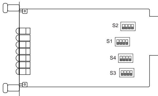
Figure 1. Model 1004ABRC Card, showing location of configuration switches.
