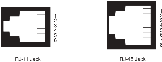
Figure 1: RJ-11 and RJ-45 Modular Pin Assignments
