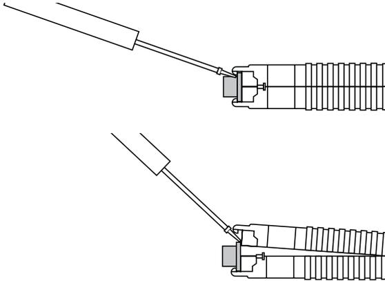
**Figure 2.** Opening the Model 1052 case
