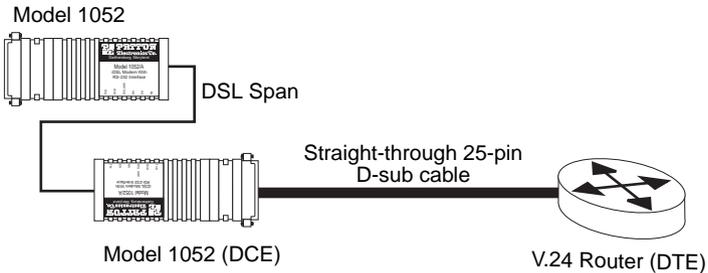
Figure 5. Connecting the Model 1052/A to an RS-232 serial DTE
