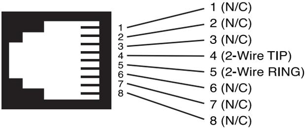
Figure 4. Model 1052 twisted pair line interface
