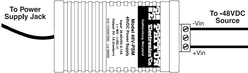
Figure 6. Connecting DC power to the 48V-PSM DC power supply
