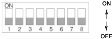
Figure 2. Close-up of DIP switches showing "ON" and "OFF" positions
