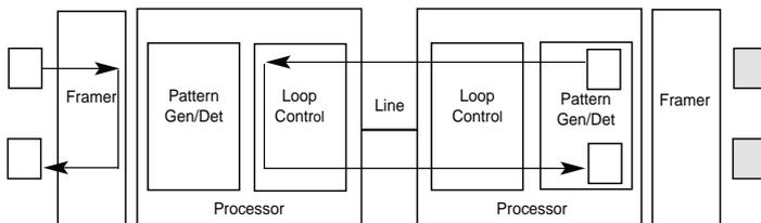
Figure 17. Block Diagram Local Loop Mode 2 with 511/511E
