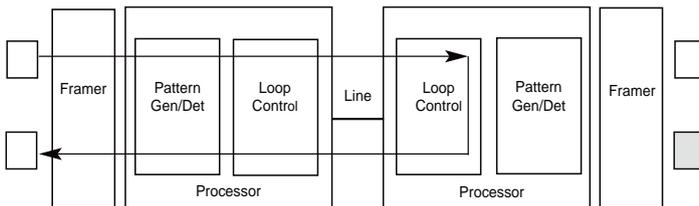
Figure 18. Block Diagram Remote Loop
