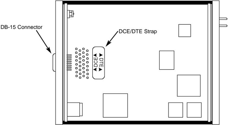
Figure 9. Setting the DCE/DTE Strap
