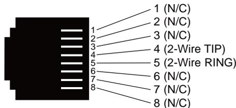
Figure 4. Model 1088 RJ-45 twisted pair line interface.
