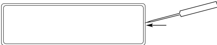
**Figure 8.** Opening the 1088 Case with a Small Screwdriver
