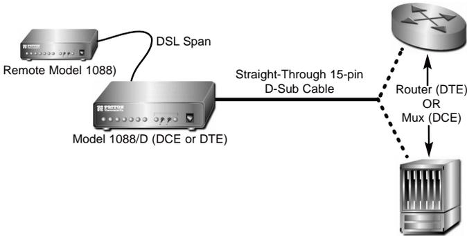
**Figure 7.** Connecting the Model 1088/D to X.21 DTE or DCE
