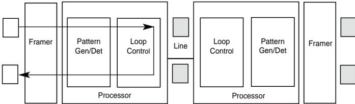
Figure 14. Block Diagram Local Loop Mode 1
