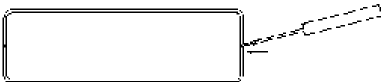
Figure 7. Opening the 1088 Case with a Small Screwdriver
