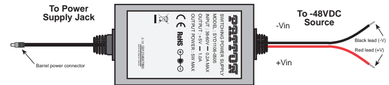
Figure 9. Connecting DC Power to the 48V-PSM DC Power Supply.
