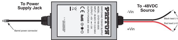
Figure 9. Connecting DC power to the 48V-PSM3 DC power supply.
