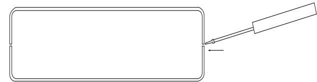
Figure 5. Using a Large Flat Blade Screwdriver to Open the Plastic Case
