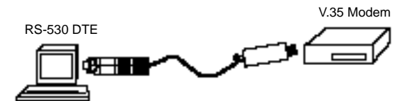
Figure 1. A common RS-530 DTE to V.35 DCE installation
