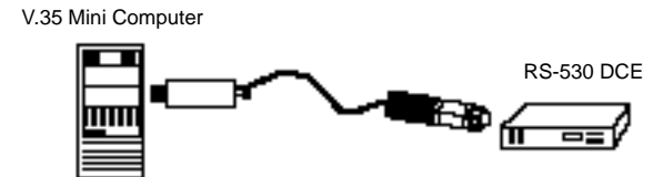
Figure 2. A common V.35 DTE to RS-530 DCE installation
