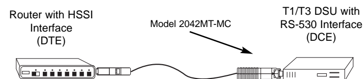
Figure 8. A Common HSSI DTE to RS-530 DCE Installation
