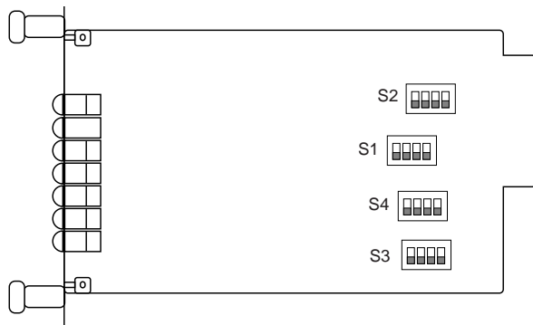
Figure 1. Model 2085RC board, showing location of configuration switches.
