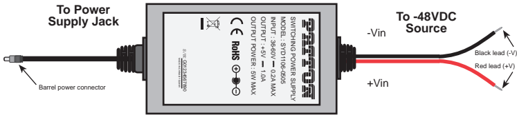
Figure 11. Connecting DC Power to the 2120 DC Power Supply
