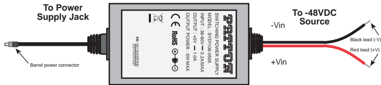
Figure 5: Connecting DC Power to the 2121/2135C DC Power Supply.
