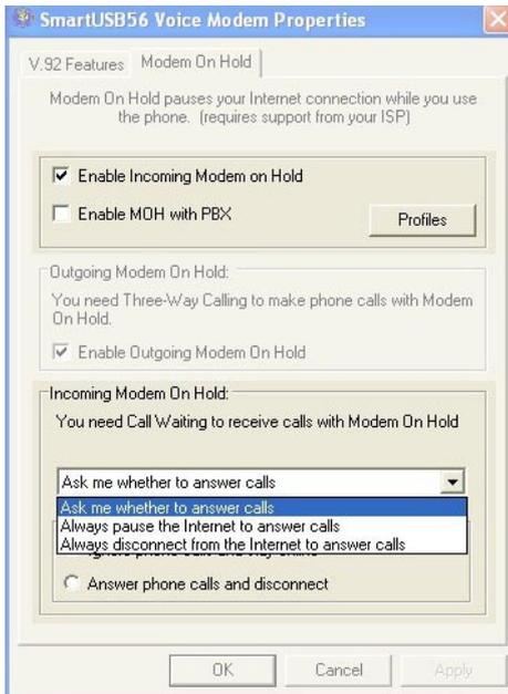
Figure 14. Modem on Hold panel
