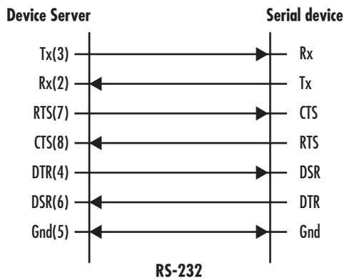
Figure 13. RS-232 wiring diagram
