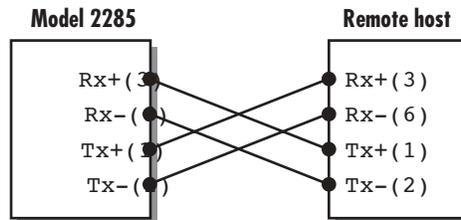
Figure 11. Ethernet direct connection using crossover Ethernet cable
