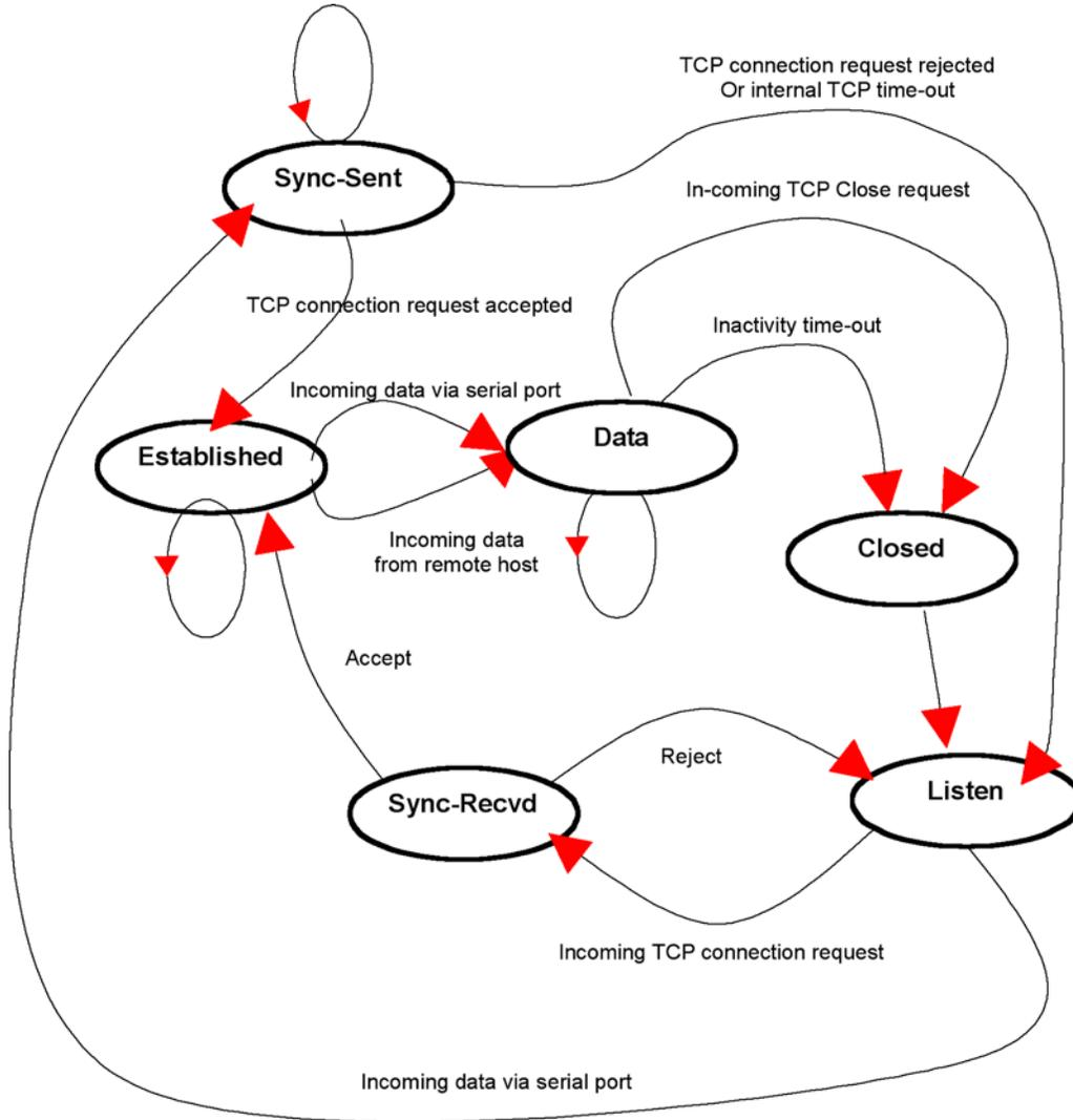
Figure 8. State Transition Diagram of TCP server/client mode
