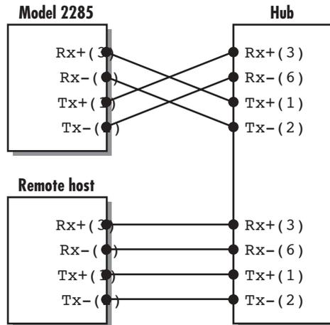
Figure 12. Ethernet connection using straight through Ethernet cable
