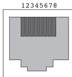
Figure 9. Pin layout of the RJ45 connector
