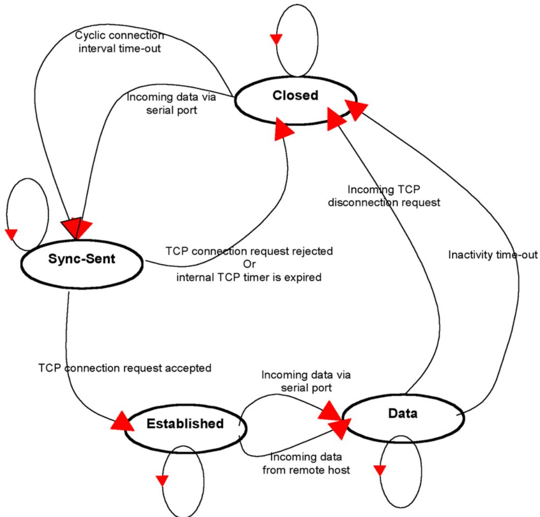
Figure 7. State Transition Diagram of TCP client mode
