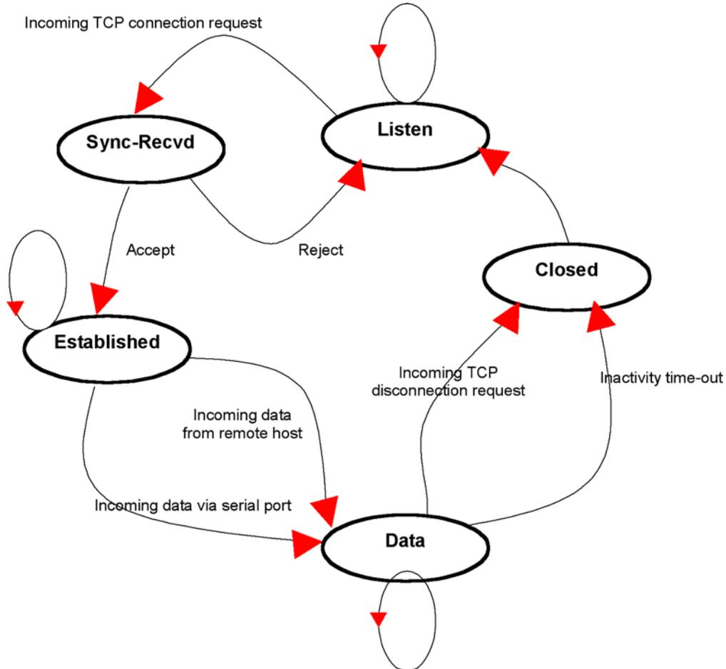
Figure 6. State Transition Diagram of TCP server mode
