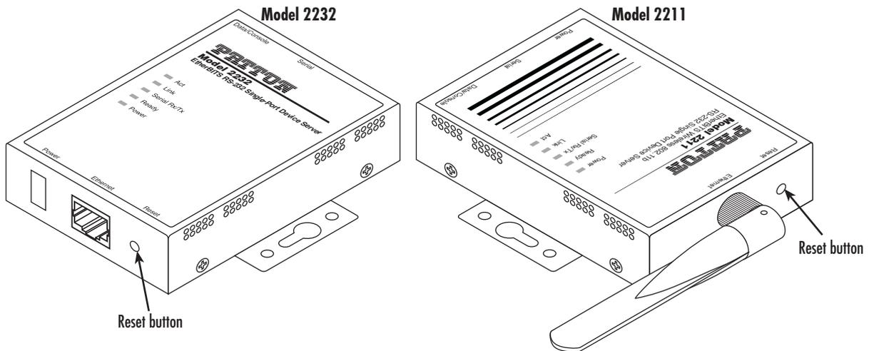
Figure 4. *Factory Reset* button location
