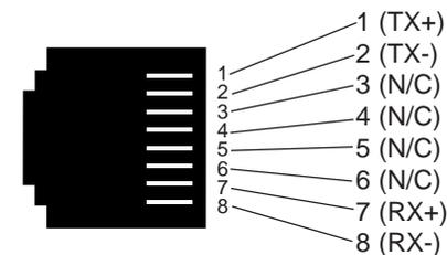
**Figure 4.** Model 2530 twisted pair line interface.
