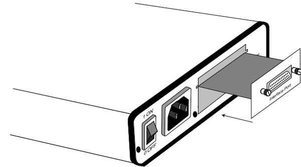
Figure 3. Installation of Model 2530 Plug-in Serial Interface Module
