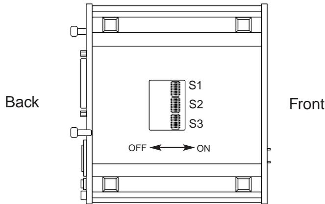
Figure 1. Underside of Model 2530, Showing Location of DIP Switches
