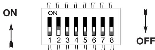
Figure 2. Close Up of Configuration Switches (all three sets are identical in appearance)
