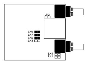
Figure 5. Jumper locations on Model 2703 PC board.
