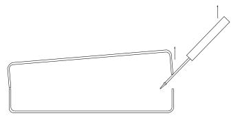
Figure 4. Opening the 2703 Case With a Small Screwdriver
