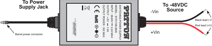
Figure 10. Connecting DC power to the 2707/I DC power supply
