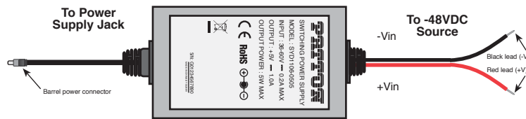
Figure 8. Connecting DC Power to the 2888 DC Power Supply
