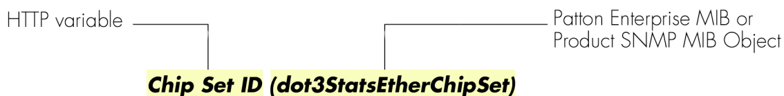
Figure 2. HTTP/HTML and SNMP object format
