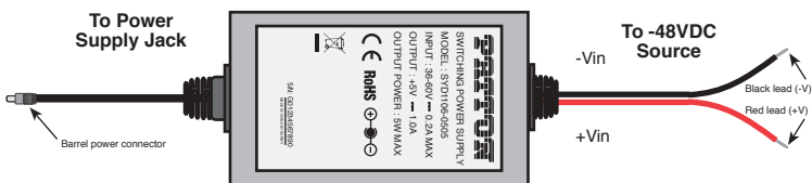
Figure 1. Connecting DC Power to the DC Power Supply
