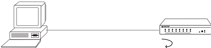
Figure 8. Local Loopback Test
