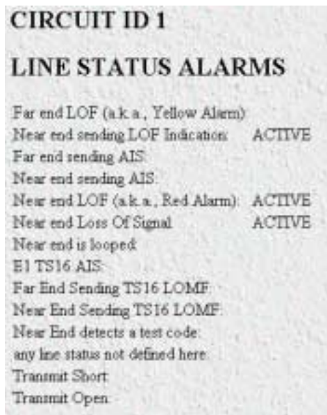
Figure 46. Line Status Alarms window
