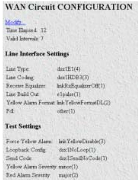
Figure 47. WAN Circuit Configuration window
