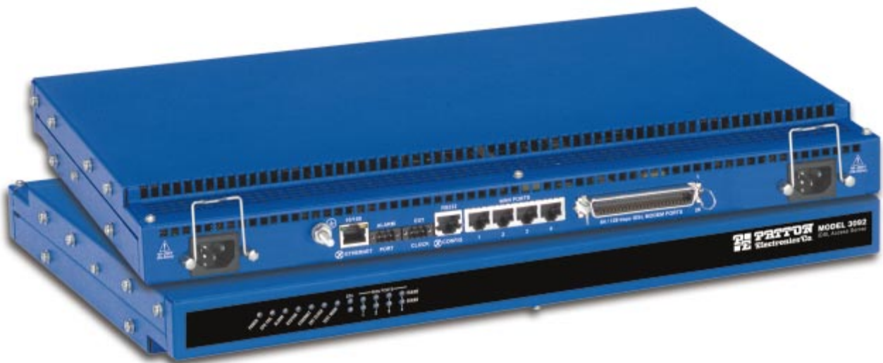
Figure 1. Model 3092 DACS (Cobalt Blue version shown)
