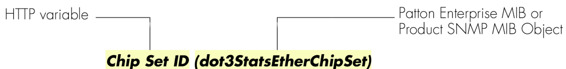
Figure 2. HTTP/HTML and SNMP object format
