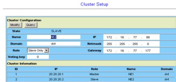
Figure 15. Cluster Configuration - Slave State
