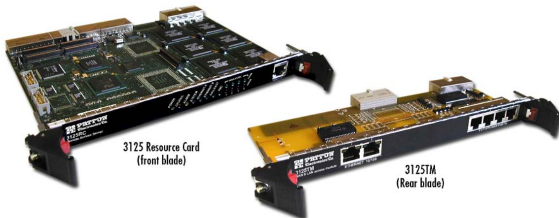
Figure 1. Model 3125 Resource Card front blade and 3125 TransitionModule rear blade
