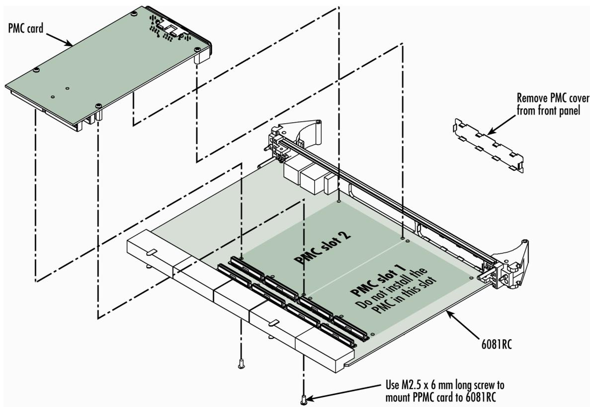
**Figure 1.** Installing the PMC Ethernet Access Module
