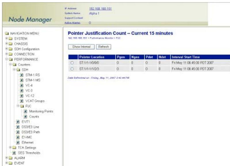
Figure 48. Displaying PM Data for PJC Counts
