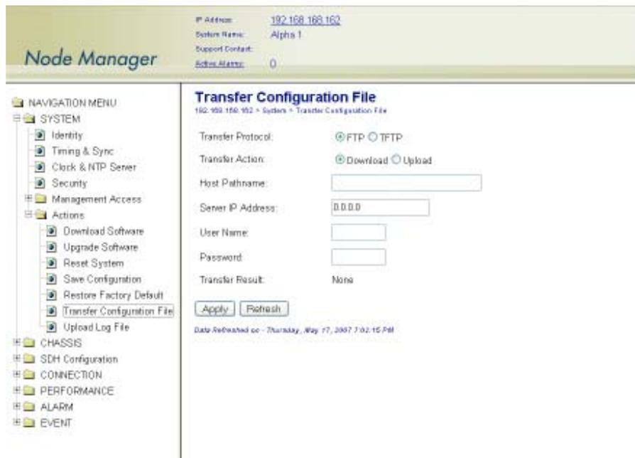
Figure 24. Transferring the System Configuration File
