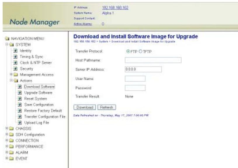
Figure 22. Downloading and Installing the System Software
