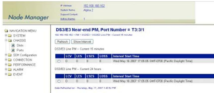
Figure 99. Displaying Current Line PM Data for DS3/E3 Ports
