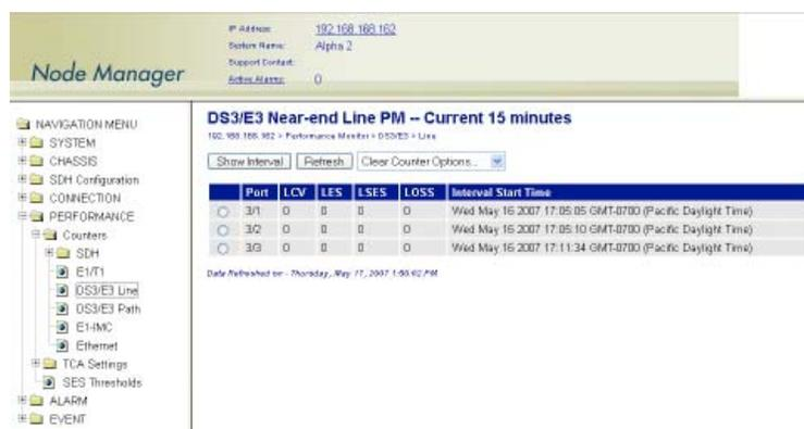
Figure 100. Displaying Current Line PM Data for All DS3/E3 Ports
