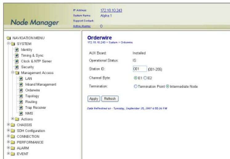
Figure 9. Configuring the Engineering Orderwire (EOW) Function
