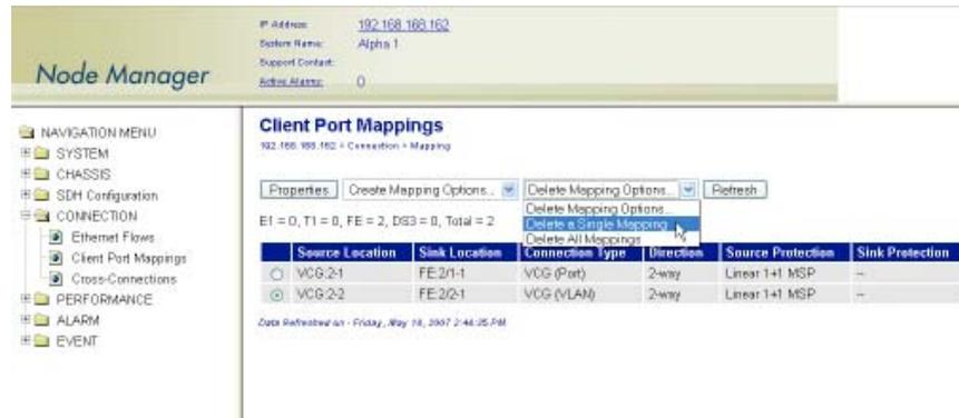
Figure 126. Removing an Ethernet Flow from a VCG
