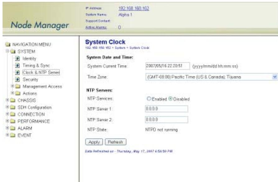
Figure 21. Configuring Access to an NTP Server
