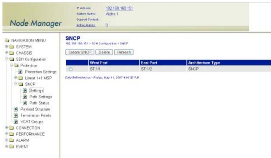
Figure 67. Configuring STM-1 Ports in SNCP Mode
