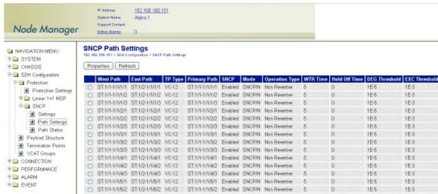
Figure 68. Displaying and Configuring the SNCP Path Settings
