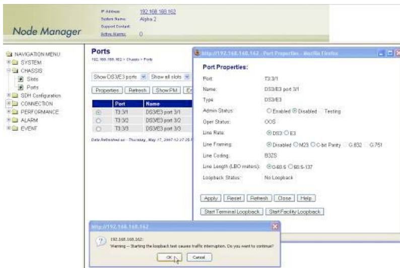
Figure 104. Activating DS3/E3 Loopback
