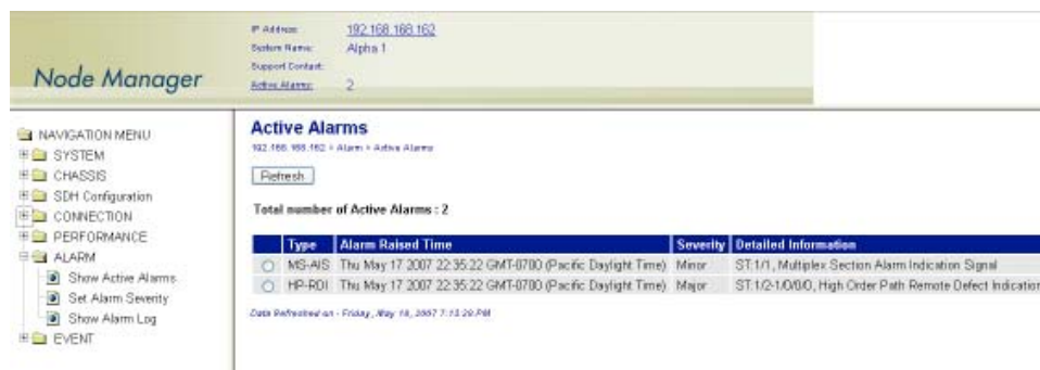
Figure 41. Displaying SDH Alarms
