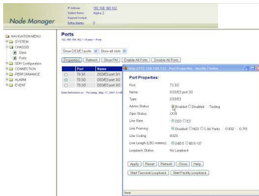
Figure 93. Enabling a DS3/E3 Port
