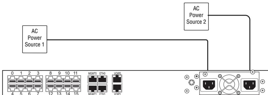
**Figure 5.** Connecting the power source
